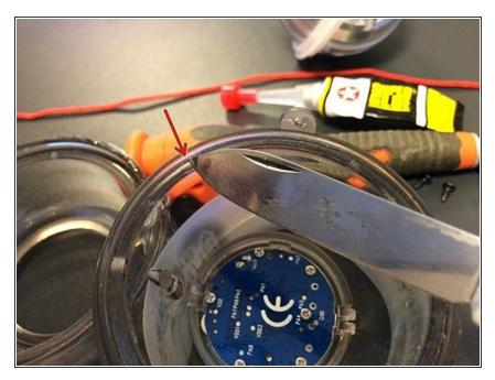
Use some sharp tool and remove surpluses, make these places as smooth as you can. From time to time put gyro back in place and roll it on both halves of housing until you'll feel it's enough.
