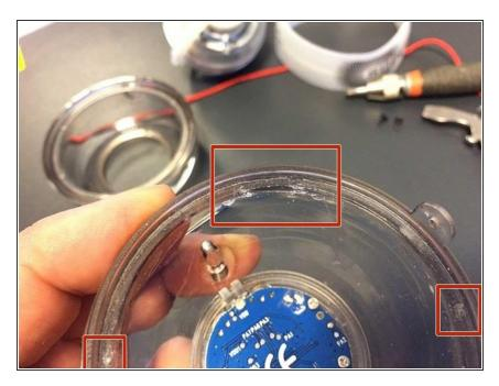
Look at these surfaces and you will find several small deflections. They were made by gyro's axis when it hit the floor. These deflections put up resistance during rolling and this is the reason it's so hard to spin device.
