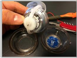
Remove gyro. It's connected to white plastic roundel which really is a part of inner bearing. It slides
