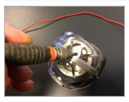
Find two small Phillips screws holding both housing halves and unscrew them.
