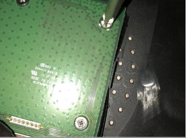
Unscrew board from plastic cover. There's a total of 4-.7 cm flat hear Philips screws.
