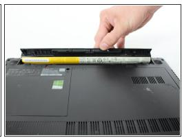
Once both switches are pulled, the battery should pop out.
