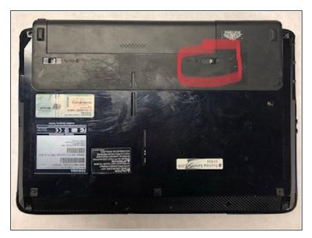
Slide locking tab above battery to open position while sliding out battery
