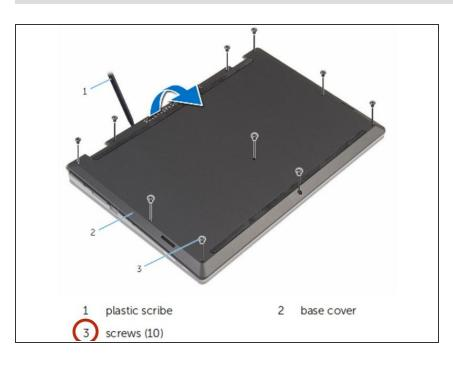
Remove the ten screws that secure the base cover to the base of the computer.
