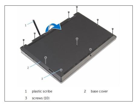
Using a plastic scribe (plastic opening tool), pry the base cover off of the base of the computer.
