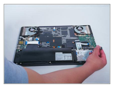
Remove the screw holding the solid state drive. Place the screw on the magnetic mat
