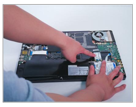
Locate the solid state drive. It is initially obscured by a connector, its okay to push away the connector to access the solid state drive.
