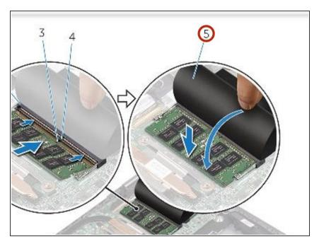
Lift the Mylar to access the memorymodule slot.
