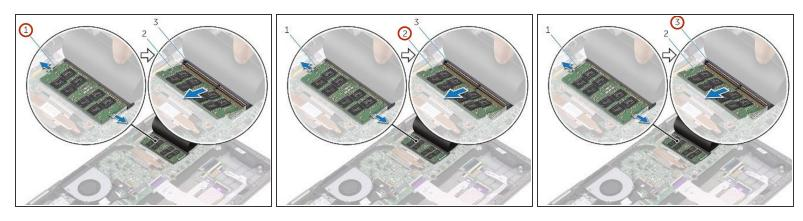
• Use your fingertips to carefully spread apart the securing-clips on each end of the memory-module slot until the memory module pops up.
