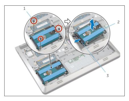
Replace the screws that secure the hard-drive assembly to the base frame.
