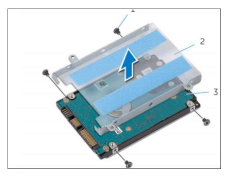
Place the hard-drive bracket on the NEW hard drive.
