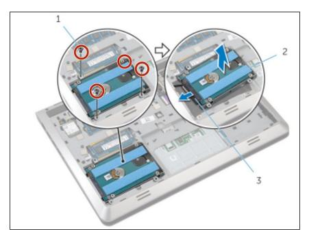
Remove the screws that secure the hard-drive assembly to the base frame.
