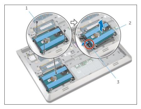
Connect the hard-drive cable to the hard drive.
