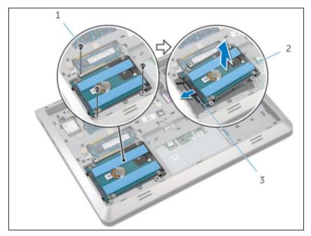
Place the hard-drive assembly in the base frame and align the screw holes on the hard-drive assembly with the screw holes on the base frame.
