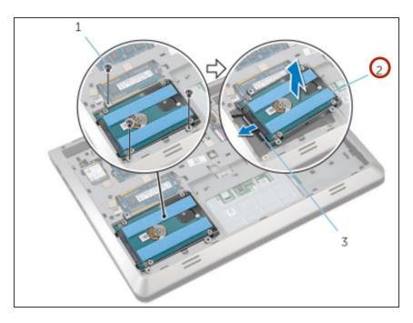
Gently lift the hard-drive assembly out of the base frame and disconnect the hard-drive cable from the hard drive.
