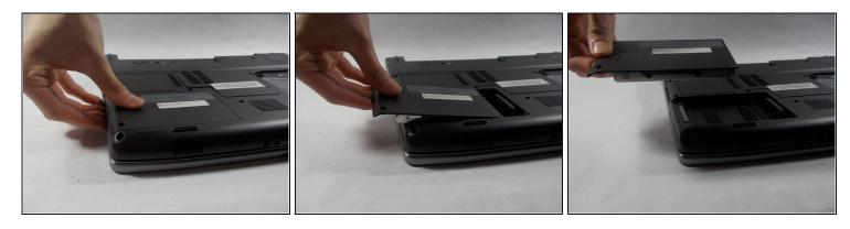
Press down firmly on the hard drive and pull leftwards.
