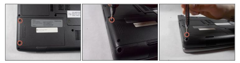
• Remove the two 6 mm Phillips #0 screws from the back of the hard drive cover.
