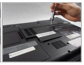
• Remove the seven 6mm screws from the back panel with a Phillips #0 screwdriver.
