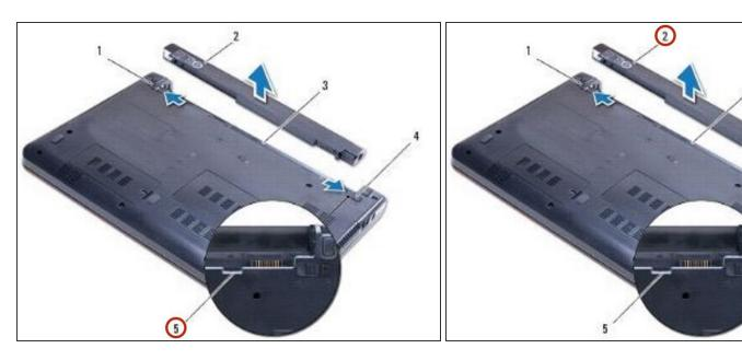
At the notch, lift the battery to remove it from the battery bay.
