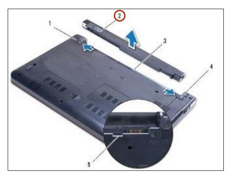
Push down on the battery to connect it to the computer.
