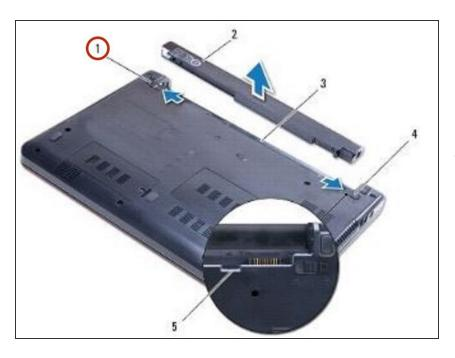
Slide the battery release latch to the unlock position. The battery release latch automatically shifts to the
