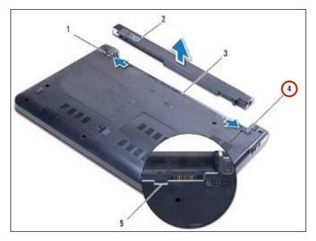
Slide the battery lock latch to the unlock position.
