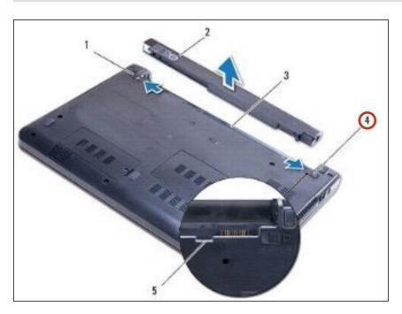
Slide the battery lock latch to the locked position.
