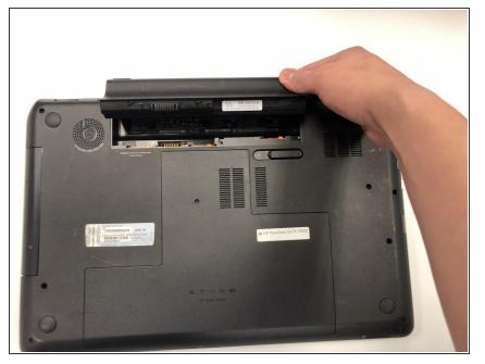
Hold the release switch all of the way to the left and your other hand to pull the battery out.
