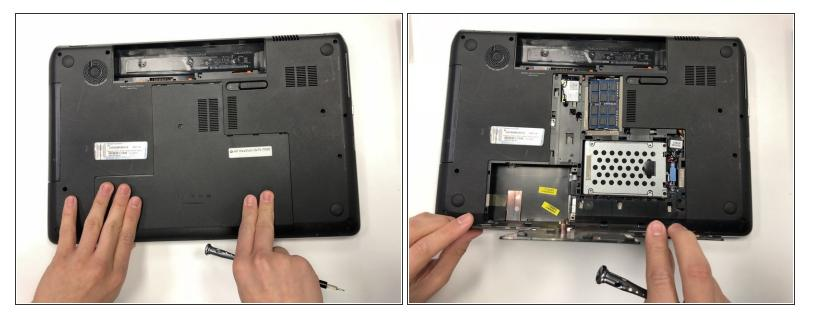
• Remove service hatch by sliding away from the computer and lifting up.
