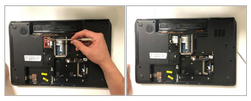
• Use the flat end of a spudger to pop off the antenna connectors.
