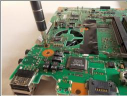
Using a Philips head size #0 remove the 3mm screw on the back of the motherboard.
