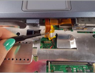
Remove the ribbon from the motherboard with a pair of tweezers.
