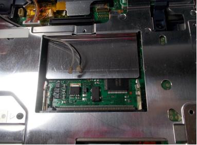
• Take out the Adapter and carefully pull the wires out from the metal casing.
