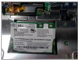
Use tweezers to remove the wires from the Adapter.
