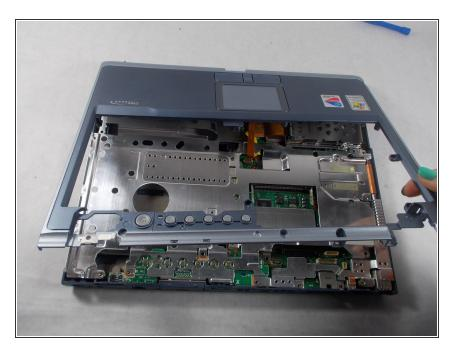
Lift up the plastic frame from the base to expose the ribbon attached to the motherboard.
