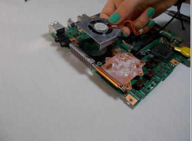
• The fan can now be removed from the motherboard.
