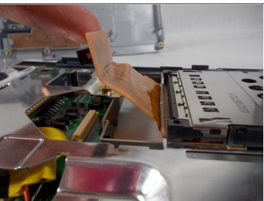
Pull the ribbon tab up and off the motherboard.
