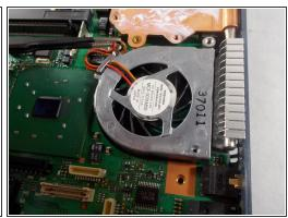
Using tweezers detach the cable from the motherboard.
