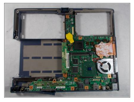
Remove the metal plate covering the motherboard.
