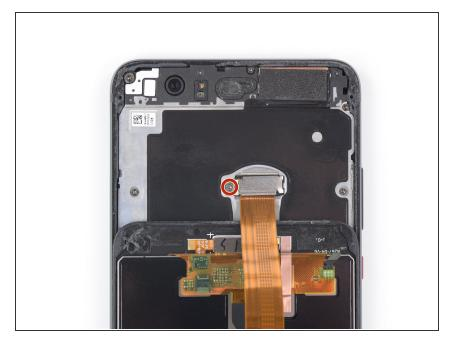
Remove the 3.3 mm-long Phillips screw securing the display flex connector bracket.
