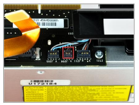
Disconnect the speaker cable connector from the interconnect board by lifting its connector up off the socket on the board.
