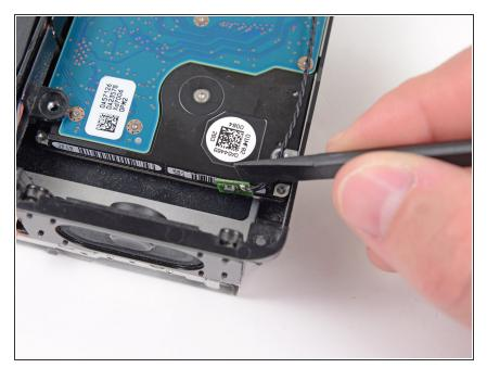
• Use the flat end of a spudger to pry the hard drive thermal sensor board off the adhesive securing it to the side of the hard drive.
