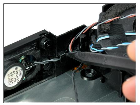
• Use the tip of a spudger to de-route the speaker cable from the clip on the internal frame.
