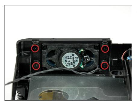
Remove the four shouldered Phillips screws securing the speaker assembly to the internal frame.
