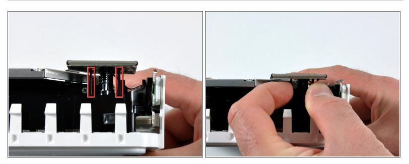
• Slightly squeeze the two retaining arms toward each other and lift the AirPort antenna off its post.
