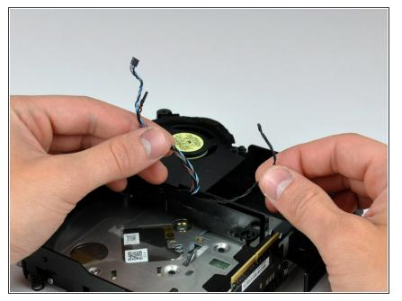
• De-route the speaker cable from within the channel in the internal frame.
