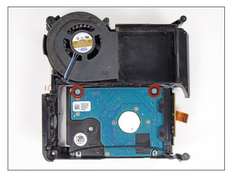
Remove the two Phillips screws connecting the underside of the hard drive to the internal frame.
