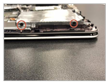
Lift up the hard drive and remove the two Phillips #0 screws that hold the hard drive to the case.
