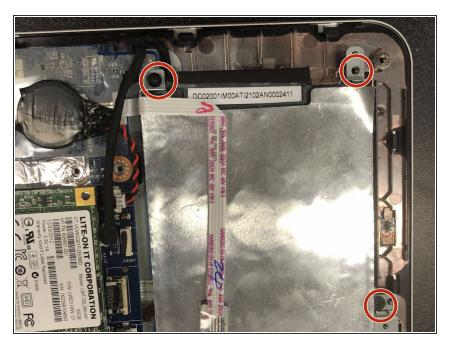
Remove the three Phillips #0 screws that secure the hard drive to the laptop.
