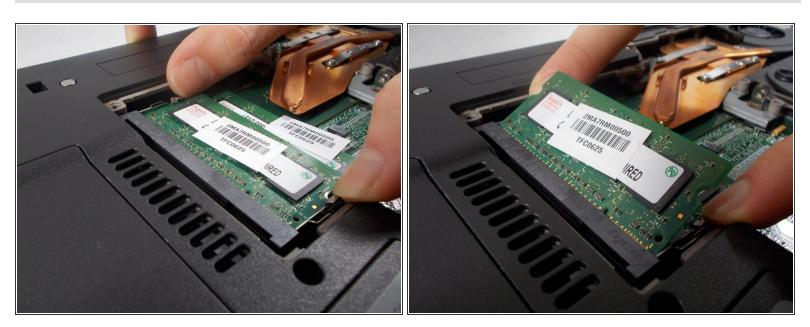
Push the two metal tabs (holding the module in place) apart in order to release it.
