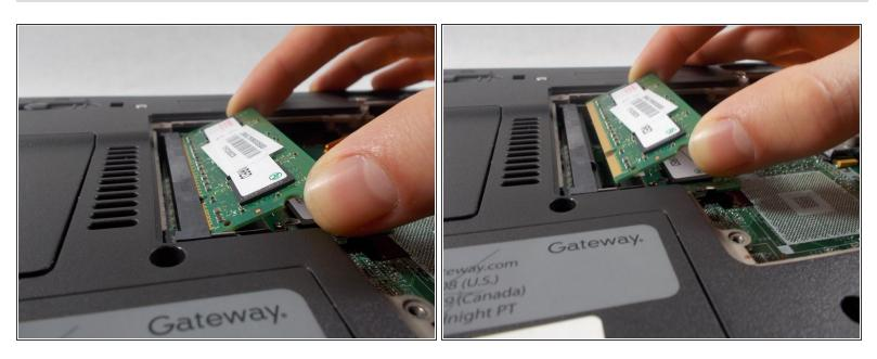
Pull the ram out of the motherboard at a 45 degree angle.
