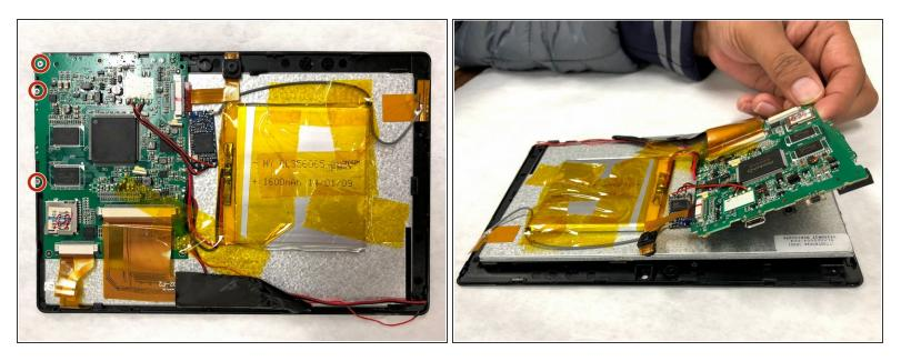
Remove the three 4 mm JIS #0 screws to release the PCB board.
