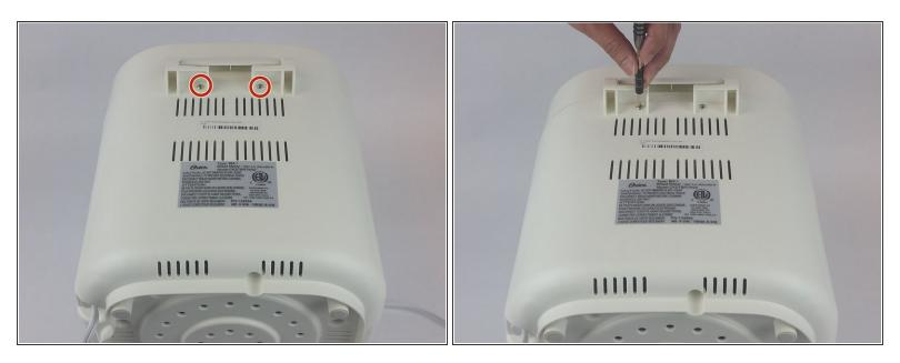
• Remove the two 11mm Phillips #1 screws from the back of the device.
