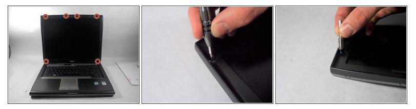
• Unscrew and remove the 6 6mm screws that were under the rubber pieces using a Phillips #1.
