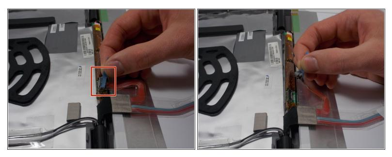
• Pull on the blue tag sticking out at the bottom of the screen and disconnect the wire.
