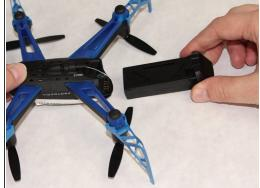
Slide the battery pack out of the drone. When replacing be mindful of the antenna as it is easily crushed.
