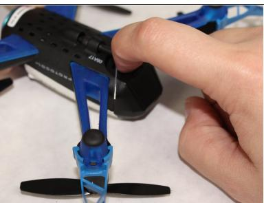
Use either the iFixit opening tool or your fingers to pry open the drone battery.
