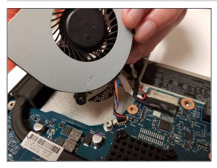
Be mindful of wires, the final step is to unplug the fan from the motherboard, at the base of red and blue wires.
