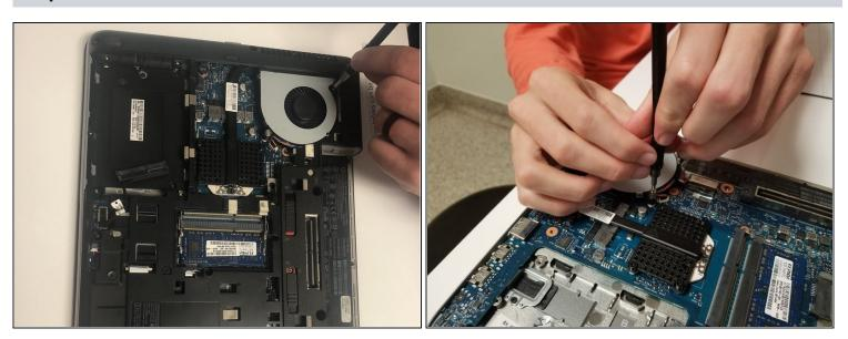
• Using a J1 head for your screwdriver, remove the 4 surrounding screws.
