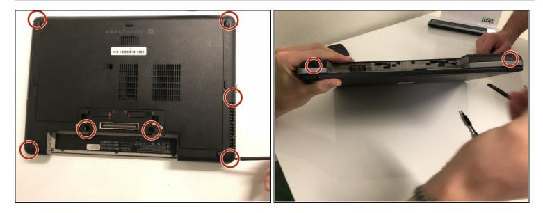
• Remove the nine screws that keep the back cover secured using the T5 Torx screwdriver.
