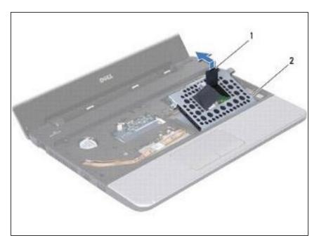
Push the hard drive assembly towards the left until it is fully connected to the interposer.
