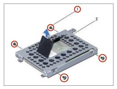
Remove the four screws that secure the hard drive bracket to the hard drive and remove the hard drive bracket.
