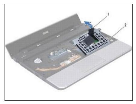
Place the hard drive assembly in the hard drive compartment.
