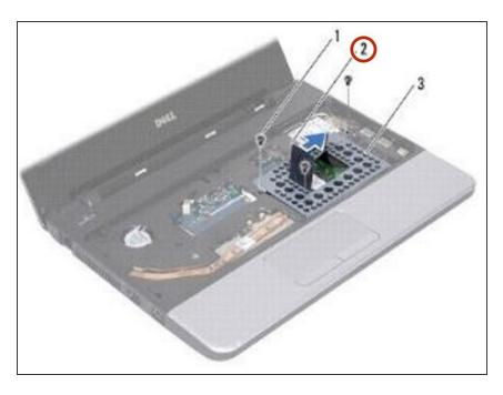
Pull the pull-tab on the hard drive bracket towards the right to disconnect the hard drive assembly from the interposer.
