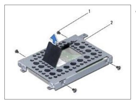
Replace the hard drive bracket and the four screws that secure the NEW hard drive bracket to the hard drive.
