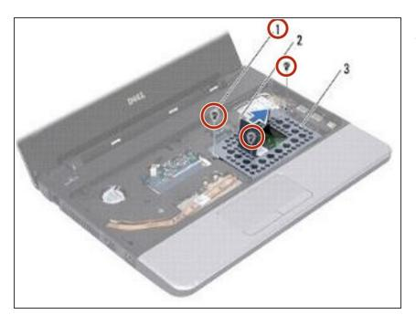
Replace the three screws that secure the hard drive assembly to the computer base.
