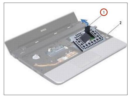
Pull the pull-tab on the hard drive bracket to lift the hard drive assembly at an angle and out of the hard drive compartment as shown in the illustration.
