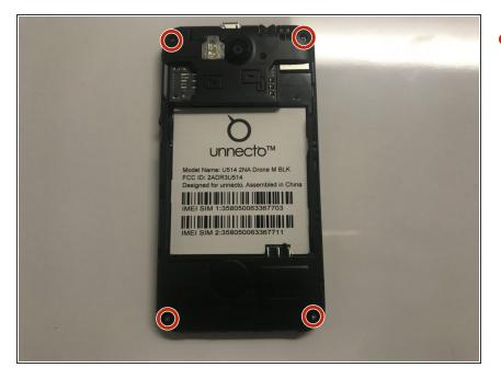
Remove the four screws on the back of the phone using a Philips 000 screwdriver
