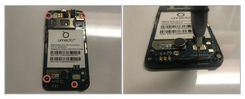
• Use a Phillips #000 screwdriver to remove the four screws that secure the motherboard.
