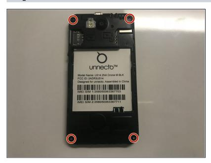
Remove the four screws on the back of the phone using a Philips 000 screwdriver
