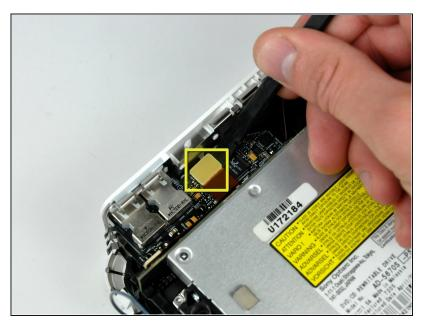
Use the flat end of a spudger to pry the audio ribbon cable connector up off the audio board.
