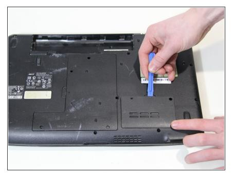
Gently pry off the panel with an opening tool. This will reveal the RAM.
