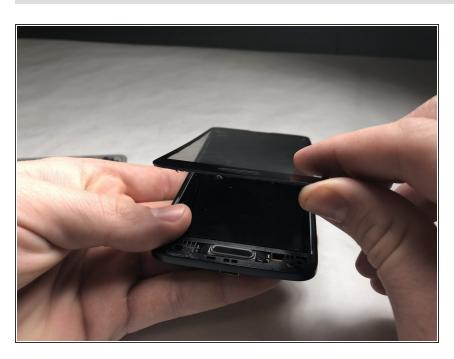
Pry the screen off after all pieces have been loosened from the adhesive.
