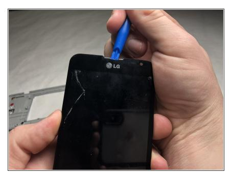
Insert the plastic opening tool between the screen and the base.
