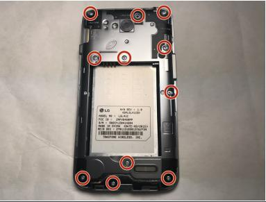
• Use a Phillips #0 screwdriver to remove the 11 mid-frame screws.
