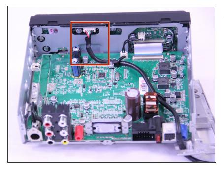
• Disconnect the USB cable from the display board.
