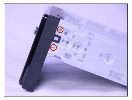
Remove the four 3.5mm Phillips #0 screws from the sides of the display.
