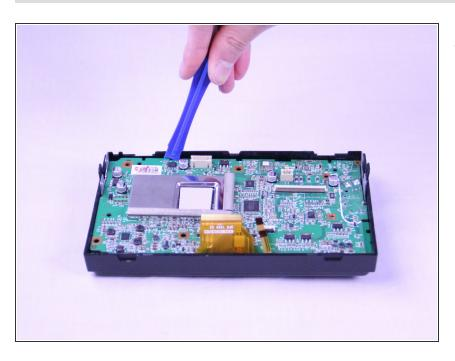
• Use a plastic opening tool to remove the display board from the radio.
