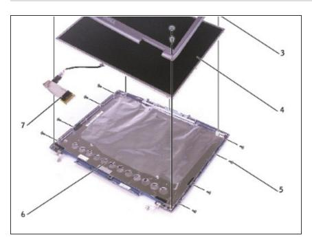
• Lift the display assembly up and out of the computer base.
