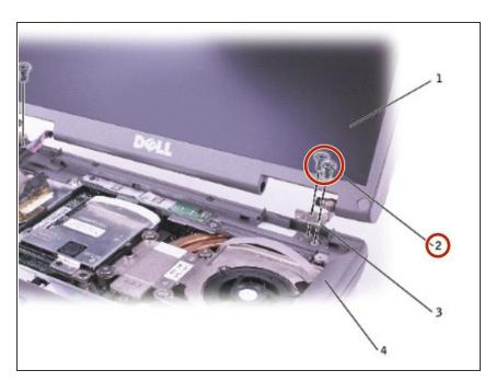
Remove the two M2.5 x 5-mm screws from each hinge bracket.
