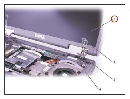
Open the display assembly approximately 180 degrees, and support the display assembly so that it does not open past this position.
