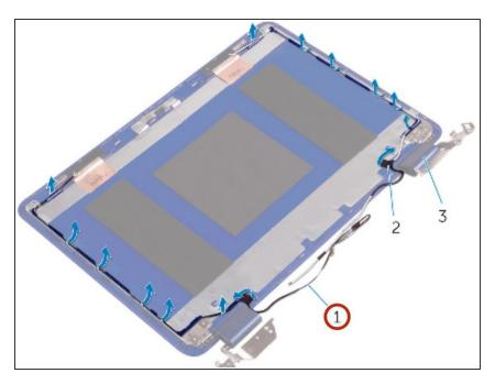
• Route the antenna cables through the routing guide on the hinge cover and secure it in place.
