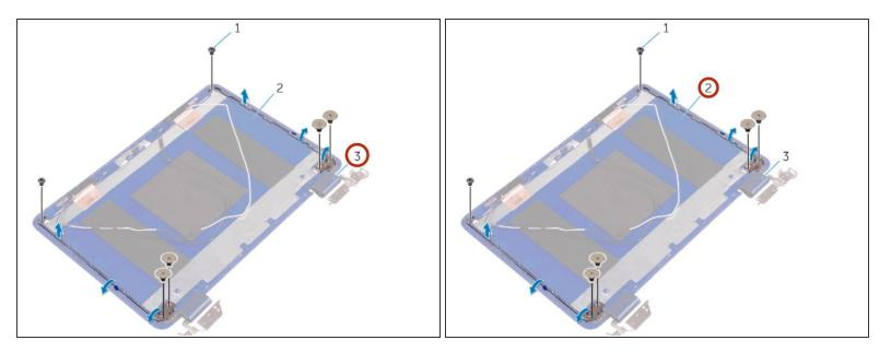
• Lift the display hinges off the display back-cover and antenna assembly.
