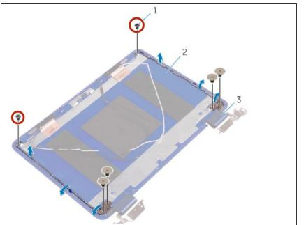
• Replace the screws that secure the display hinges to the display back-cover and antenna assembly.
