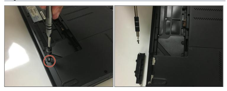
• Remove the single Phillips #0 screw that secures the hard drive cover.
