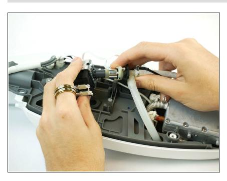
Pull apart to remove the electronic valve.
