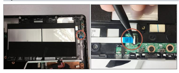
• Flip up the white part of the connector using the pointed end of a plastic spudge.
