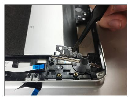
• Using <u>tweezers</u>, carefully pull out the external buttons.
