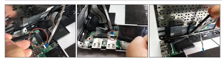
Disconnect the touchpad cable and the keyboard cable on the palm rest assembly from the motherboard using the pointed end of a plastic spudger.
