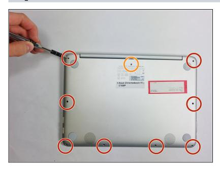
• Remove the eight 3mm bottom cover screws and one 6mm screw using a T5 screwdriver. Set apart the screw in the rear middle of the bottom cover from the the other eight screws, as it is longer than them.
