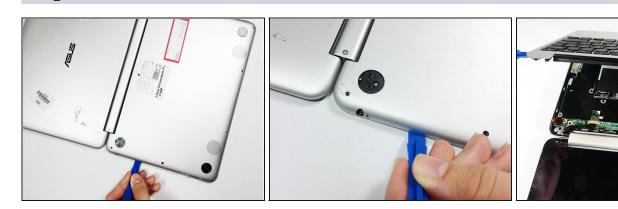
• Pry the palm rest assembly apart from the bottom cover using a spudger. This step may require a bit of elbow grease. Once the palm rest has been separated from the bottom cover, pull it away from the screen, rather than away from yourself.
