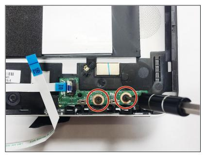
Unscrew two 2.7 mm screws using the Phillips #0 screwdriver.
