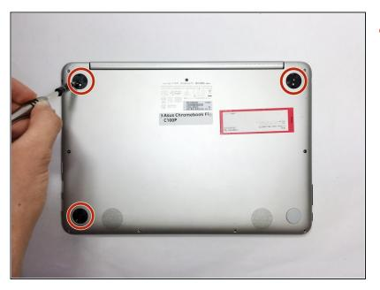
• Remove the five screws from beneath the rubber feet using a philips head screwdriver. The first 1.9mm screw is located under the front right foot, the second 1.9mm screw and third 2.3mm screw are located under the rear right foot, and the fourth and fifth 2.3mm screws are located under the rear left foot.
