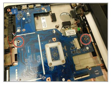
Remove the 2 screws holding the motherboard into the case of the laptop.
