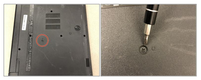
Using a Phillips #1 screwdriver, remove the small screw next to the disc engraving shown in the picture.
