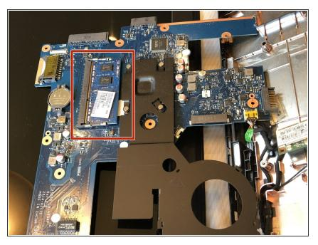
• Flip the motherboard over to access the underside revealing the RAM.
