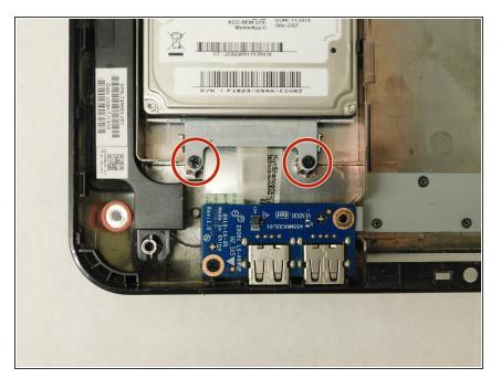
Remove the 2 black screws holding the hard drive to the computer frame.
