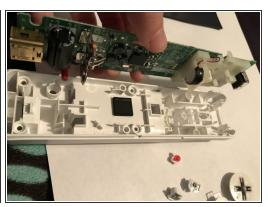
To remove the motherboard, use some tweezers to grab one of the port walls and pull upward. Be careful to not damage the inside parts though!
