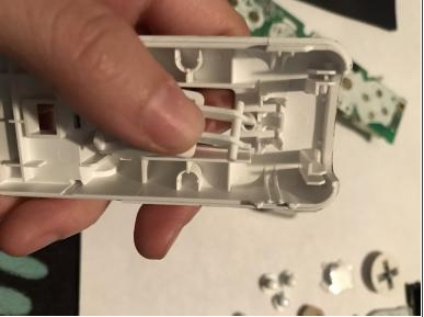
• To remove the "B" button, just push upward on it so the little pegs can pop out from the wall. You can also just get tweezer and use it to pop the pegs out.
