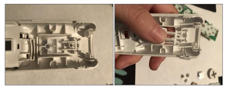
• To remove the "B" button, just push upward on it so the little pegs can pop out from the wall. You can also just get tweezer and use it to pop the pegs out.
