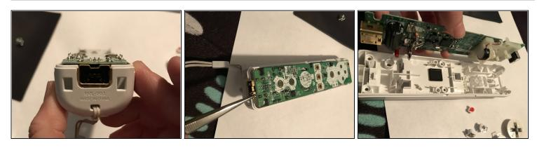
• To remove the motherboard, use some tweezers to grab one of the port walls and pull upward. Be careful to not damage the inside parts though!
