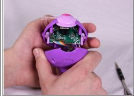
Hold the top and bottom halves of the head in each hand separately and gently pull away from each other to separate both halves.
