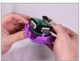
• With the head in hand, place thumbs on the screens and press gently inside and upwards to lift the screen and motherboard out from the head.
