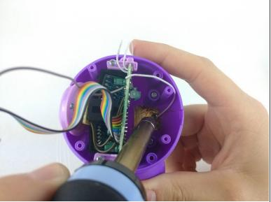
• Using a soldering iron, de-solder the wire from the gold contact sheet.
