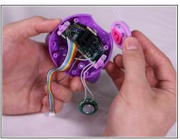
With the top half of the head in hand, push the nose in and away from the rest of the head to remove the nose.
