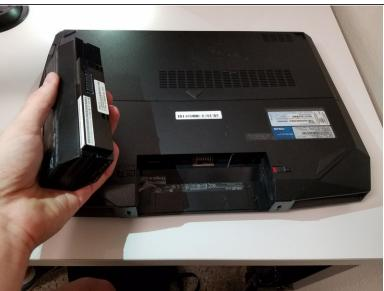
Push and hold the left switch, then pull the battery out.
