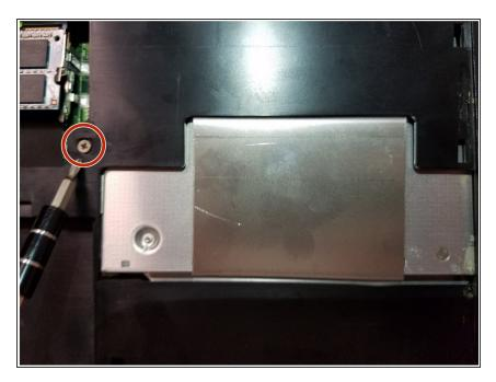
Remove the single 7mm Phillips #0 screw holding the hard drive in place.
