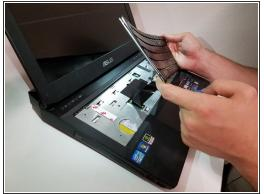
Insert a spudger, or plastic opening tool, into these five slots and pry upwards to pop up the keyboard.
