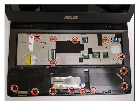
Remove the fourteen Phillips #0 screws.
