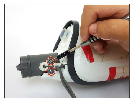
Remove the two 12.0 mm Phillips head #2 screws that hold the power cord to the device.
