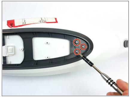
Remove the three 12.0 mm Philips head #2 screws connected to the dark grey plastic trim.
