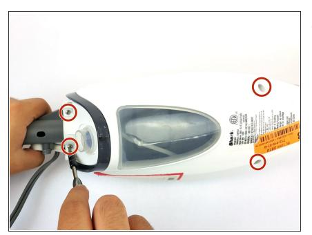
Remove the four 16.0 mm T10 Torx screws located on the back of the mop.
