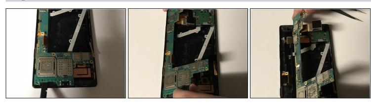
Use a spudger to pry up the bottom end of the motherboard, then pull it out.
