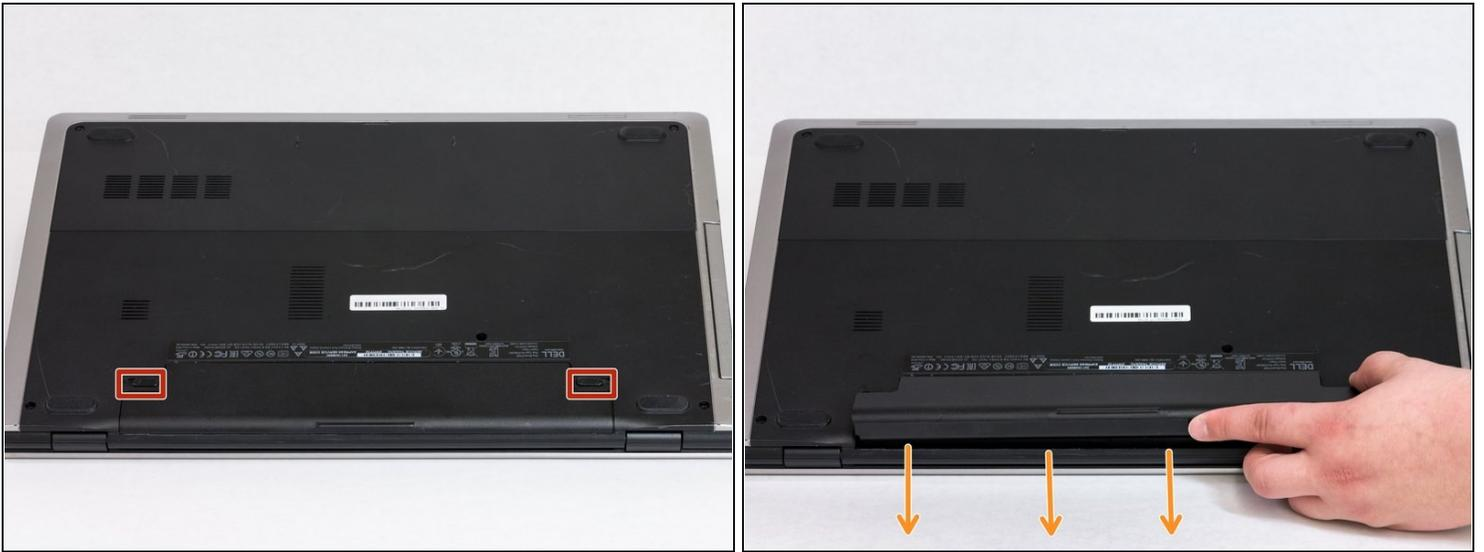
① First carefully turn the laptop over so you can access the battery.
