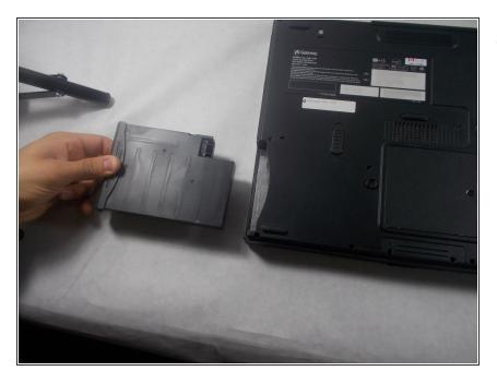
To fully free the battery it is necessary to firmly grasp the battery and give it a firm tug.
