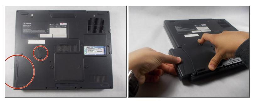
• The next step is to simultaneously push up on the battery release button and to pull out on the battery itself. If this is not done simultaneously then the battery will not budge.
