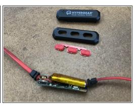
with some thin pliers or a blade pry open the button case the 2 pieces should come off with easy
