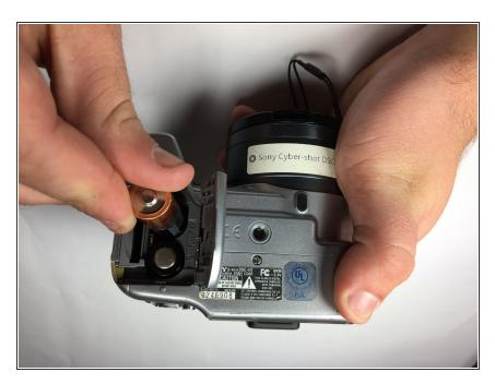
Power down the camera and remove the batteries.
