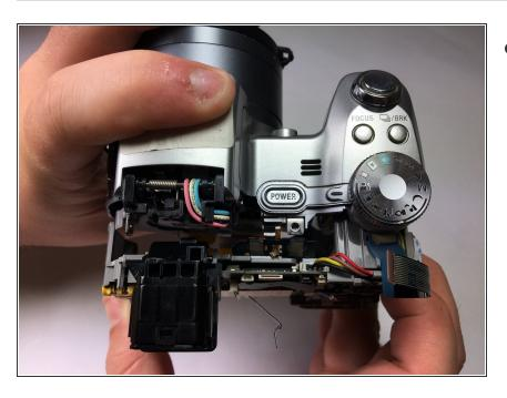
Remove the motherboard and battery pack unit.
