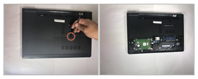
Place the plastic spudger in the slot. Using the flat side of the spudger pry the back panel upward and off.
