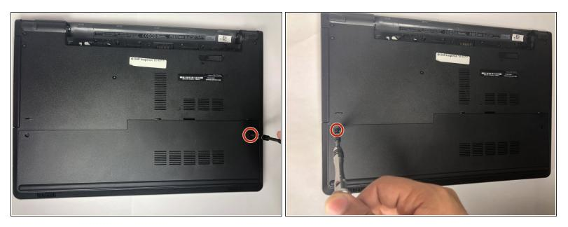
Use a Phillips #1 screwdriver to remove the two 2.5x8mm screws on the back panel.
