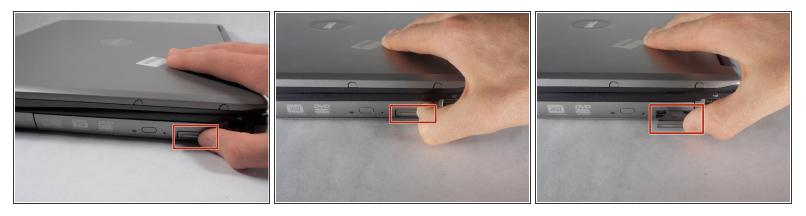
remove the CD ROM Drive: push the indicated button in towards the laptop and release. The button will pop out.
