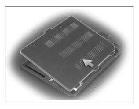
loosen the captive screws on the memory module cover, and then remove the memory module cover.
