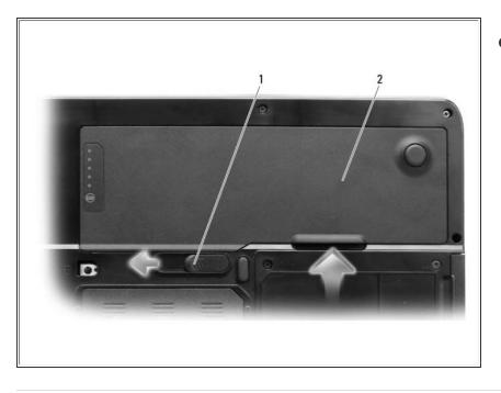
Slide and hold the battery-bay latch release on the bottom of the computer, and then lift the battery from the bay.
