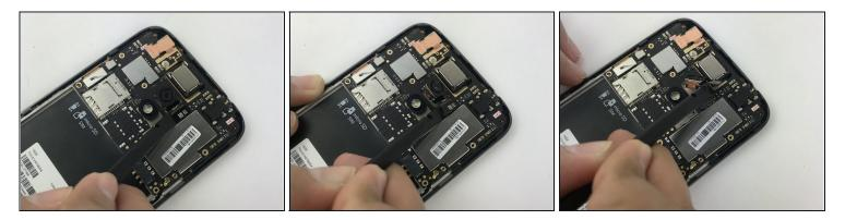
• Use the flat end of a spudger to disconnect the rear-facing camera connector from its socket on the mother board.
