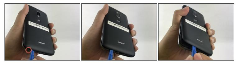
• Open case with a plastic opening tool that has the same size as the divot located at the bottom left of the phone. If you don't have an opening tool, use your finger nails.
