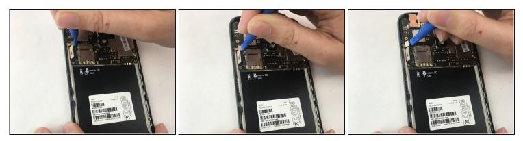
• Pry up the next connector located right on top of the previous one.
