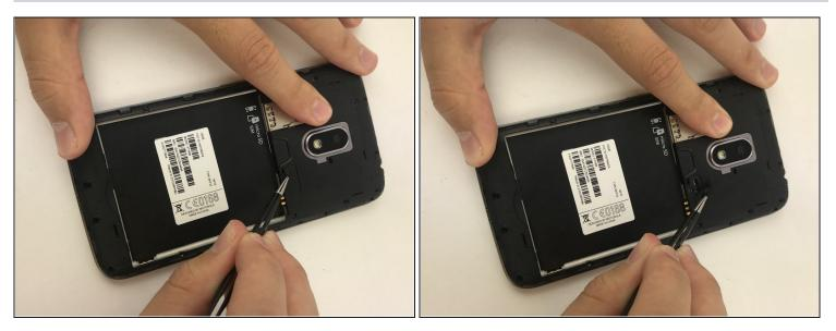
• Remove the small silicon cover at the bottom right of the camera using tweezers.
