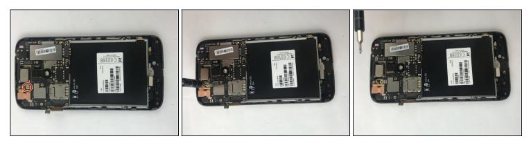
• Using the Phillips screwdriver, remove the screw that's found next to the speaker on the top left of the phone.
