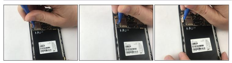
• Using an opening tool, pry up one of the connectors to the left of where the sim card was located.
