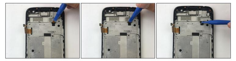
• Peel up the small tape that's connected to the screen with a plastic opening tool.
