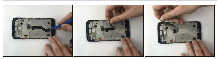
• Peel the flexible black cable using a plastic opening tool and or your fingers.
