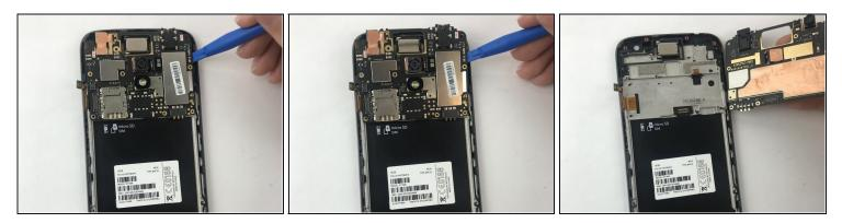
• Using the plastic opening tool, carefully pry up the motherboard.
