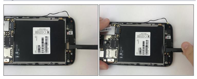
• Use the flat end of a spudger to pry up on the connector at the bottom of the battery space.
